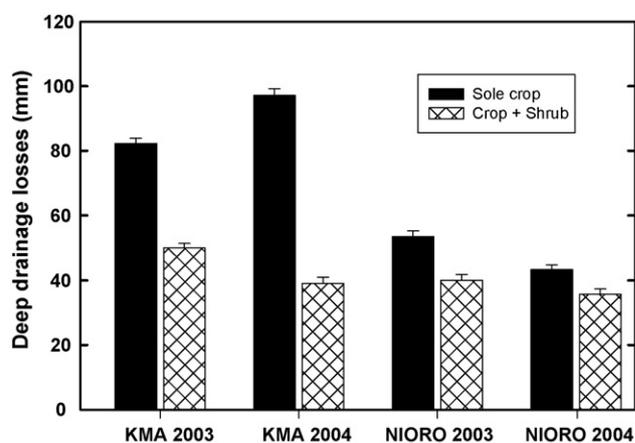
**Fig. 8 – Cumulative deep drainage water losses below the potential maximum root zone in sandy soil for both sites with millet in 2003 and peanut in 2004.**
