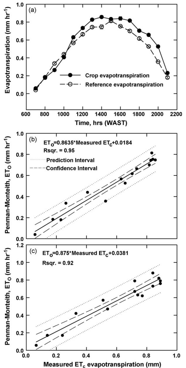
Fig. 6 – Measured and modeled  $ET$  dynamics at KMA (a and b); Niuro (c) sites, September 2004.
