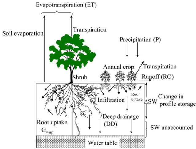
Fig. 1 – Plot water balance components.
