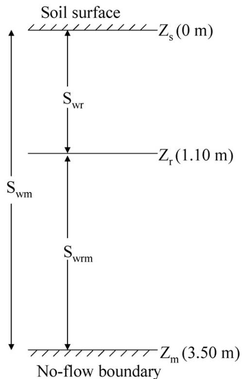
**Fig. 2 – Conceptual schematic for deep drainage estimation in sole-crop plots. The no-flow boundary is only applicable during the dry season.**
