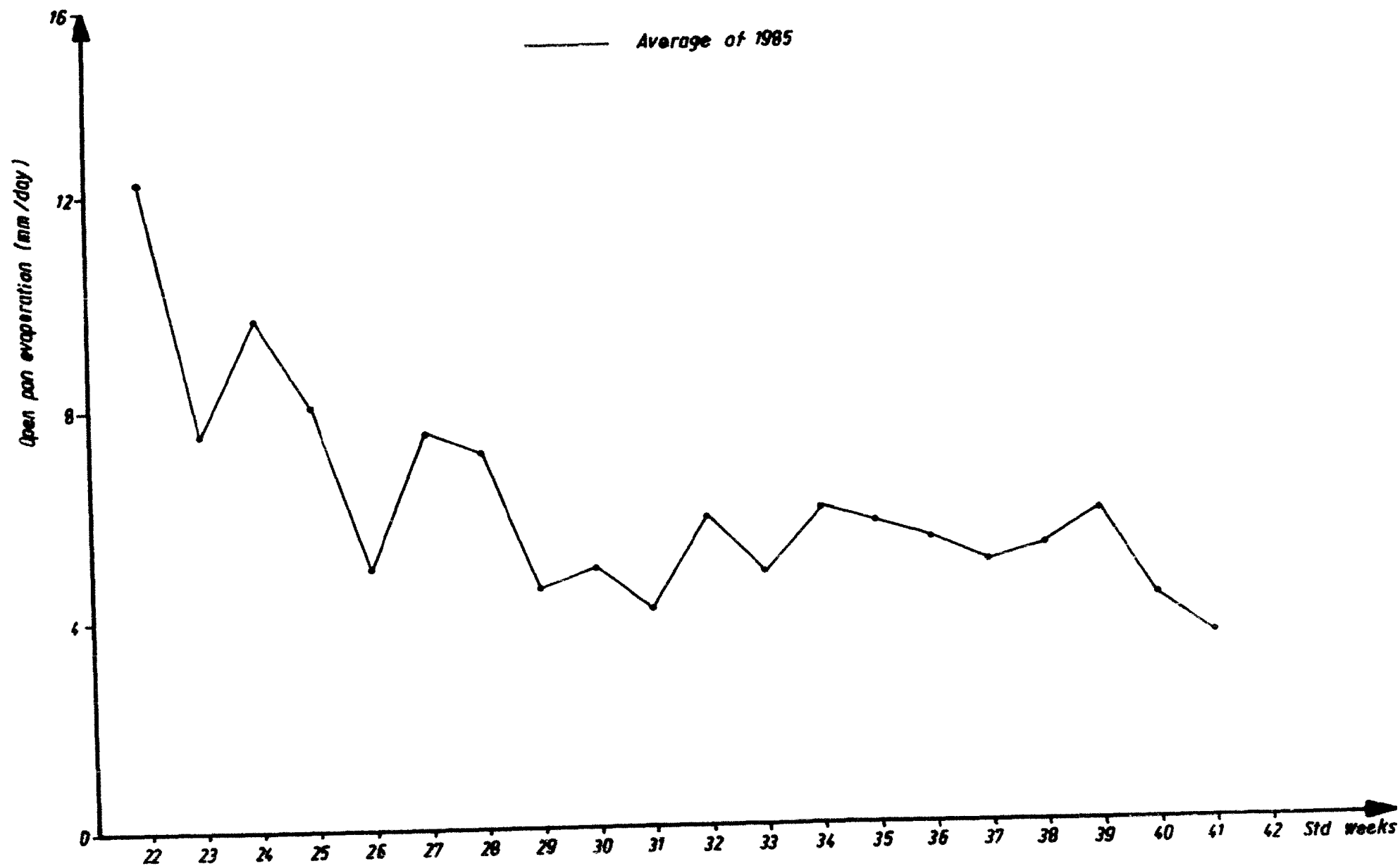
Fig 2 : Average weekly open pan evaporation at ICRISAT Center during the rainy season (1985)
